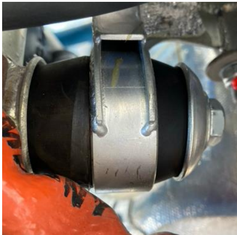
Figure 3 – Unseated rubber mount
